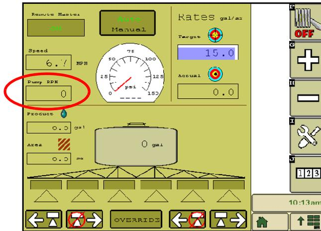
The current pump RPM is displayed in this area when a Pump RPM Cal value is entered. Refer to *Pump RPM Cal* section on page 18 to set the Pump RPM Cal value.
