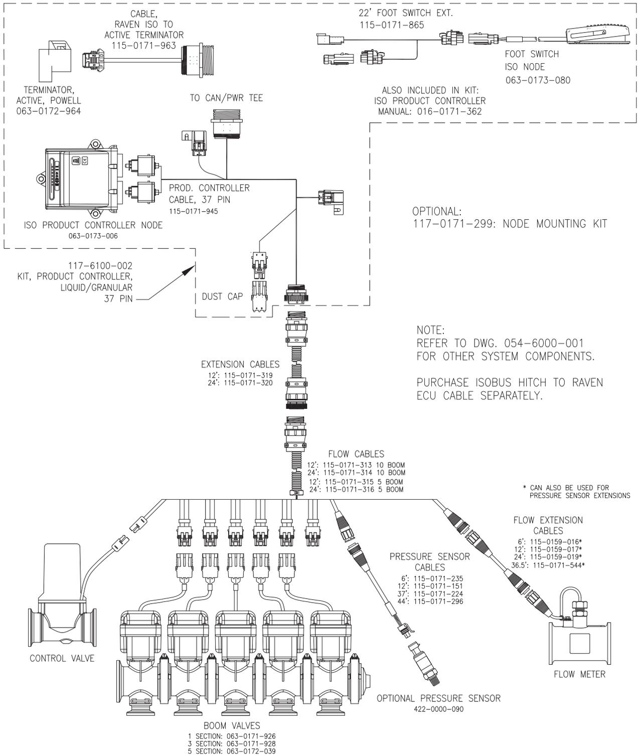
FIGURE 5. ISOBUS Liquid Product Control System (22-pin Product Cable)
