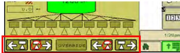
To disable sections from the left or right side of the implement, select the corresponding “OFF” button. Each time the “OFF” button is selected, the furthest enabled section on the corresponding side of the implement will be disabled. To toggle sections back on, select the corresponding “ON” button.
