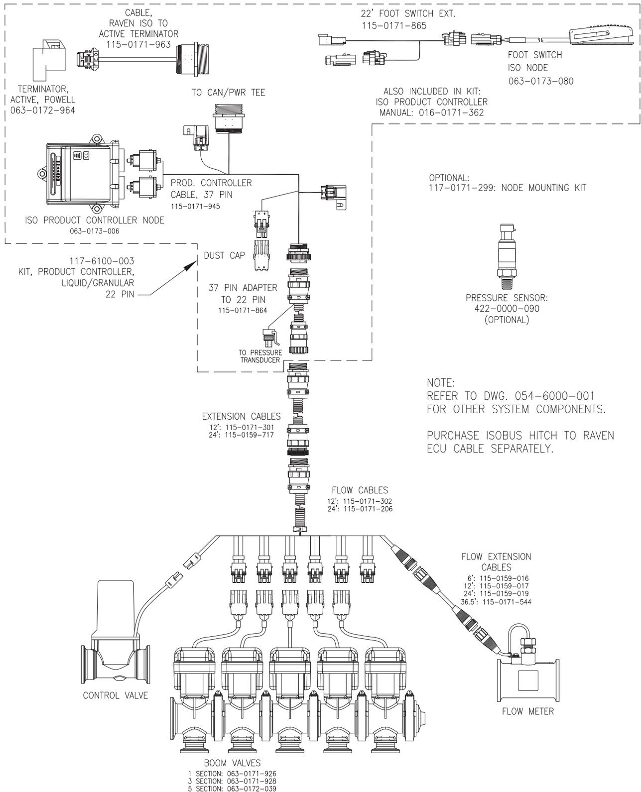
**FIGURE 6. ISOBUS Granular Product Control System (22-pin Product Cable)**
