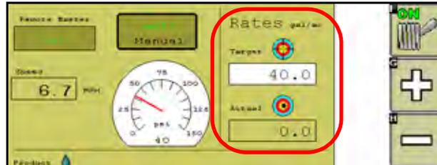
**Target Rate.** Select the target value to enter the target rate for the current application (i.e. 15 gallons per acre or 140 liters per hectare).
