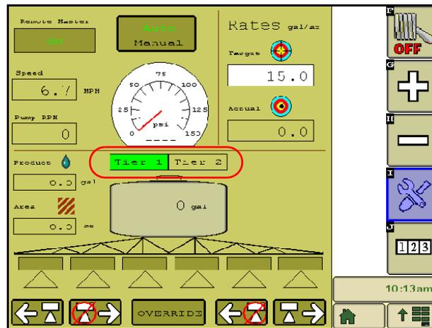
Above the tank volume display, a tiered boom status display will indicate tier 1 and tier 2 status. The tier stats will be displayed only if the tiered boom settings were entered. Refer to the *Tiered Boom Settings* section on page 19 for further information on setting up tiered booms.
