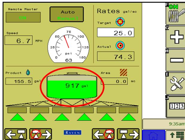
**Note:** The tank volume value must be entered in the same units used for the meter cal value. Be sure to adjust the entered tank volume using the same units or calibration as the meter cal and target rate settings. For anhydrous ammonia ( $NH_3$ ), the recommended values is pounds [kilograms] of anhydrous ammonia ( $NH_3$ ).
