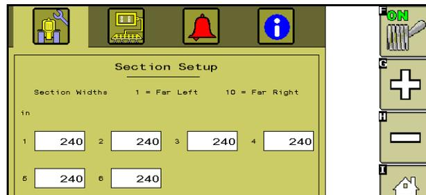
**Note:** Section measurements should be programmed into the VT display using the same units (e.g. inches, centimeters) selected in the options or settings on the VT display. Refer to the operation manual for the specific VT display to configure the display units.
