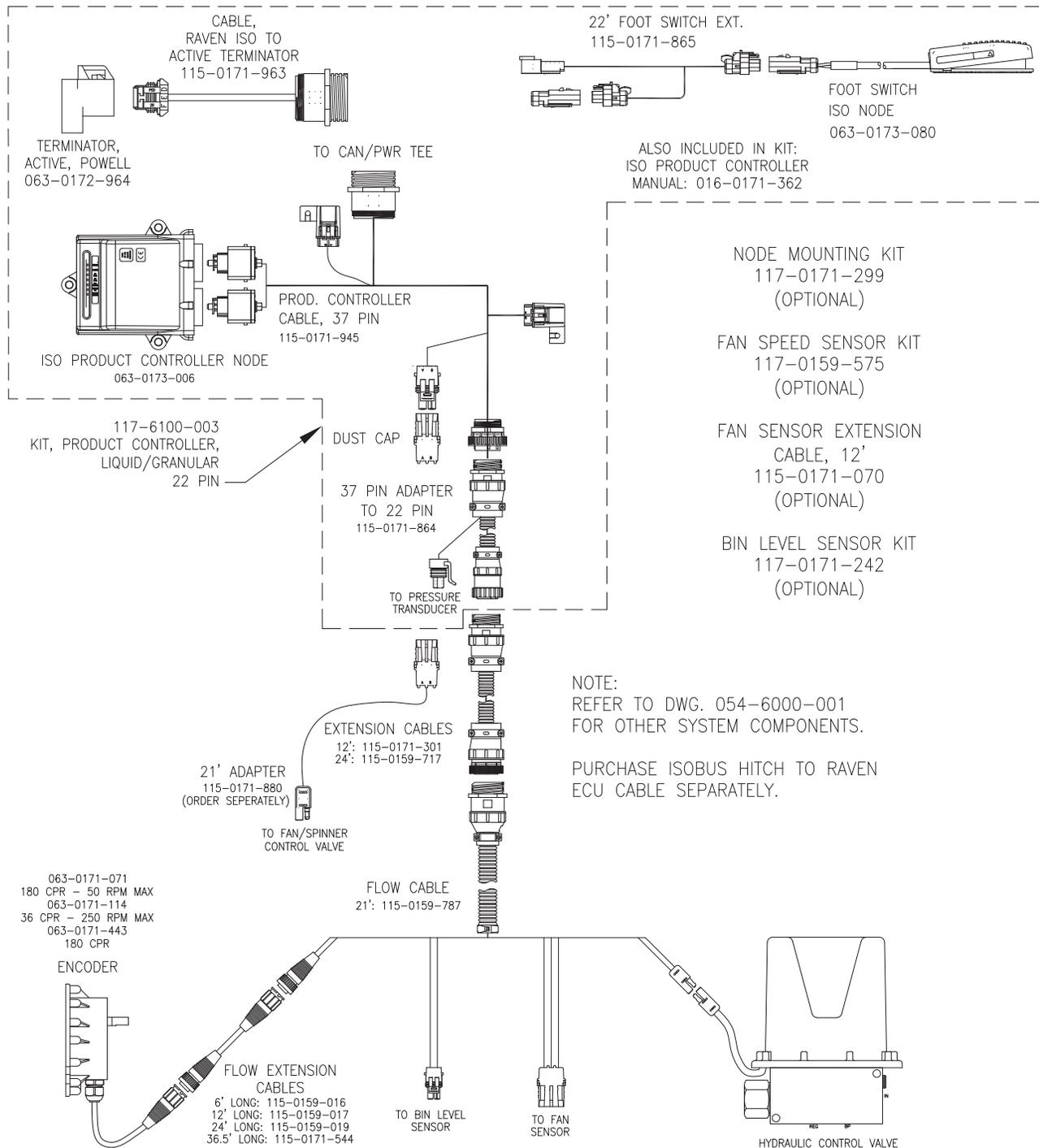
FIGURE 7. ISOBUS AccuFlow HP (3 Section Bar)
