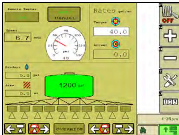
From the product control home screen, the machine operator can monitor and control the following aspects of the product control system:
