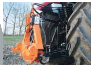
Solid adaptor frame with side-shift
